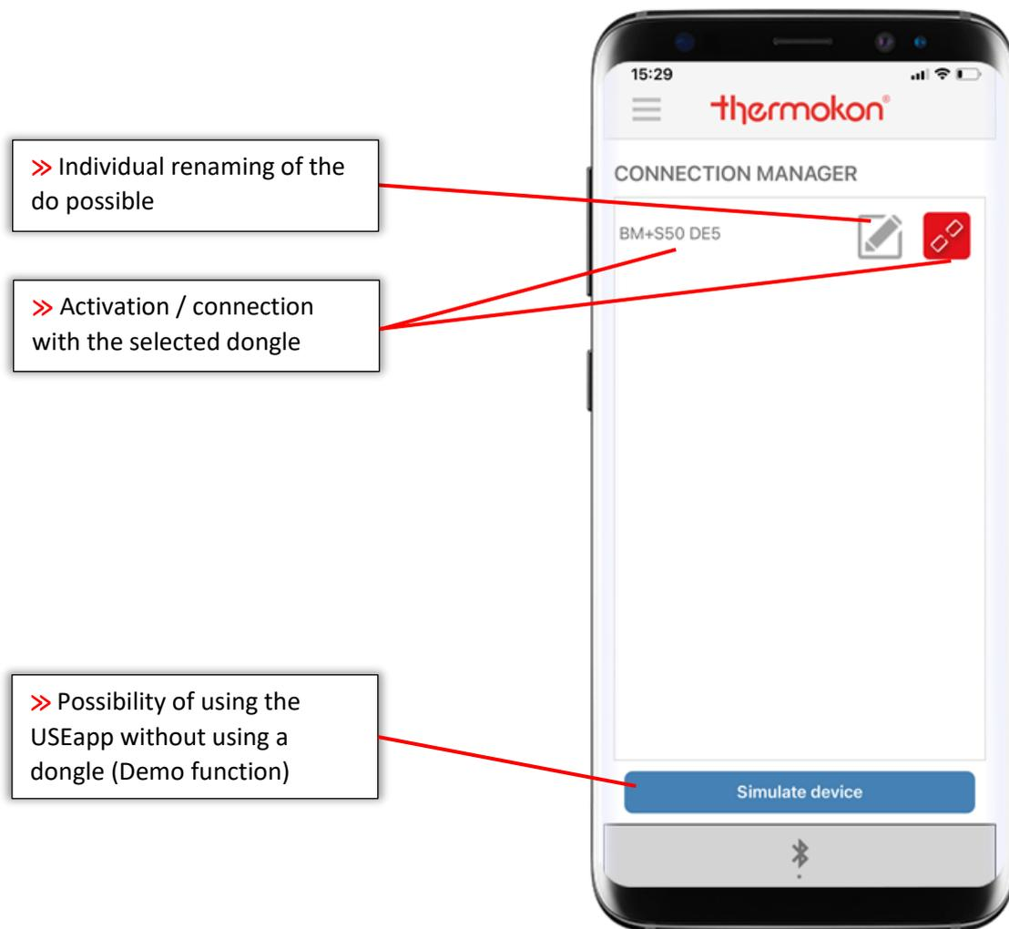
Communication with the sensor is established via the connection manager. All Bluetooth dongles available in the near distance are identified and listed in the overview. Each dongle is listed with the ID of the respective dongle. Using the small **pen icon**, it is possible to rename the dongles to create a clear identification. A simple click on the name of a dongle is all that is needed to connect it. The data are then read and the app automatically switches to the Home / Status overview.
