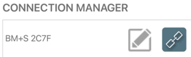
When you click on the address or name of the dongle, the connection to the device is established. Reading the data takes a few seconds. After reading the data, the app automatically jumps to the status overview.
