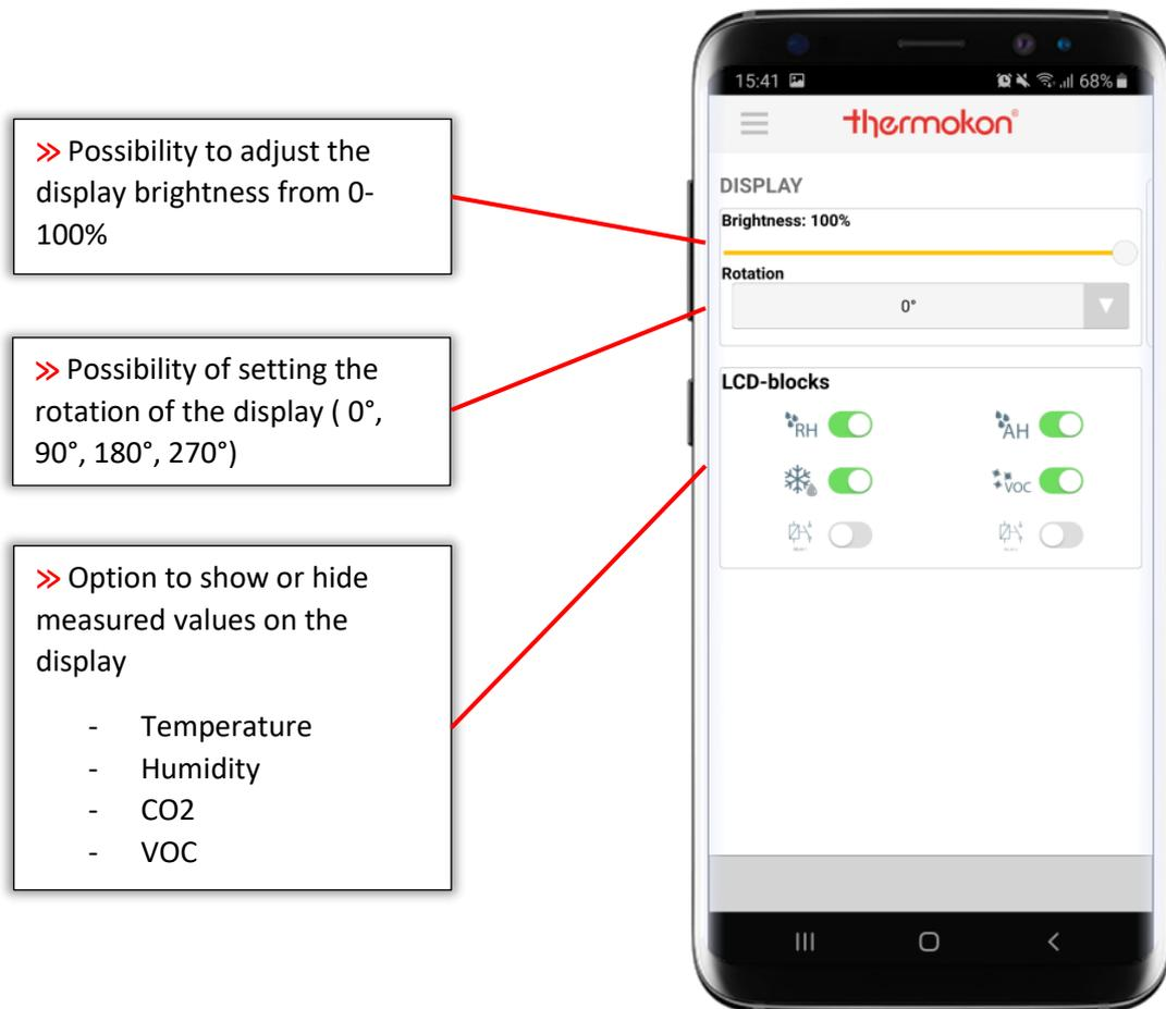
**Brightness:** Slider to change the LCD brightness. All sensors are delivered ex works with the maximum display brightness (100%).
