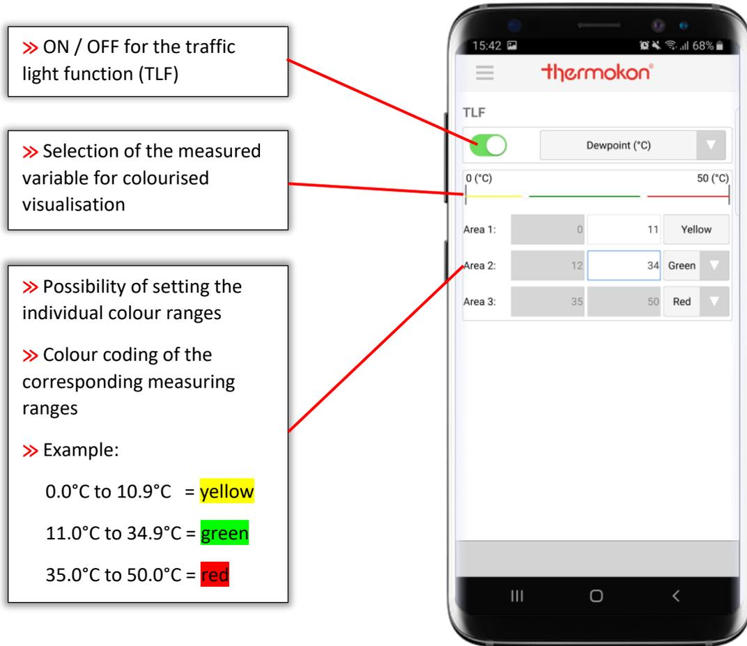
**TLF Slider:** This slider is used to activate the Traffic Light Function (TLF). With the TLF function active, a measured variable can be visualised in the display in different colours. Depending on the setting, the backlight of the display changes, when thresholds are exceeded.
