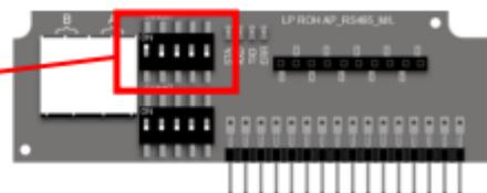
In addition, the USEapp displays all Modbus settings, such as transmission rate, address (DIP), Modbus, parity and firmware version of the Modbus plug-in PCB. These parameters are configured via the second DIP-switch on the Modbus board.
