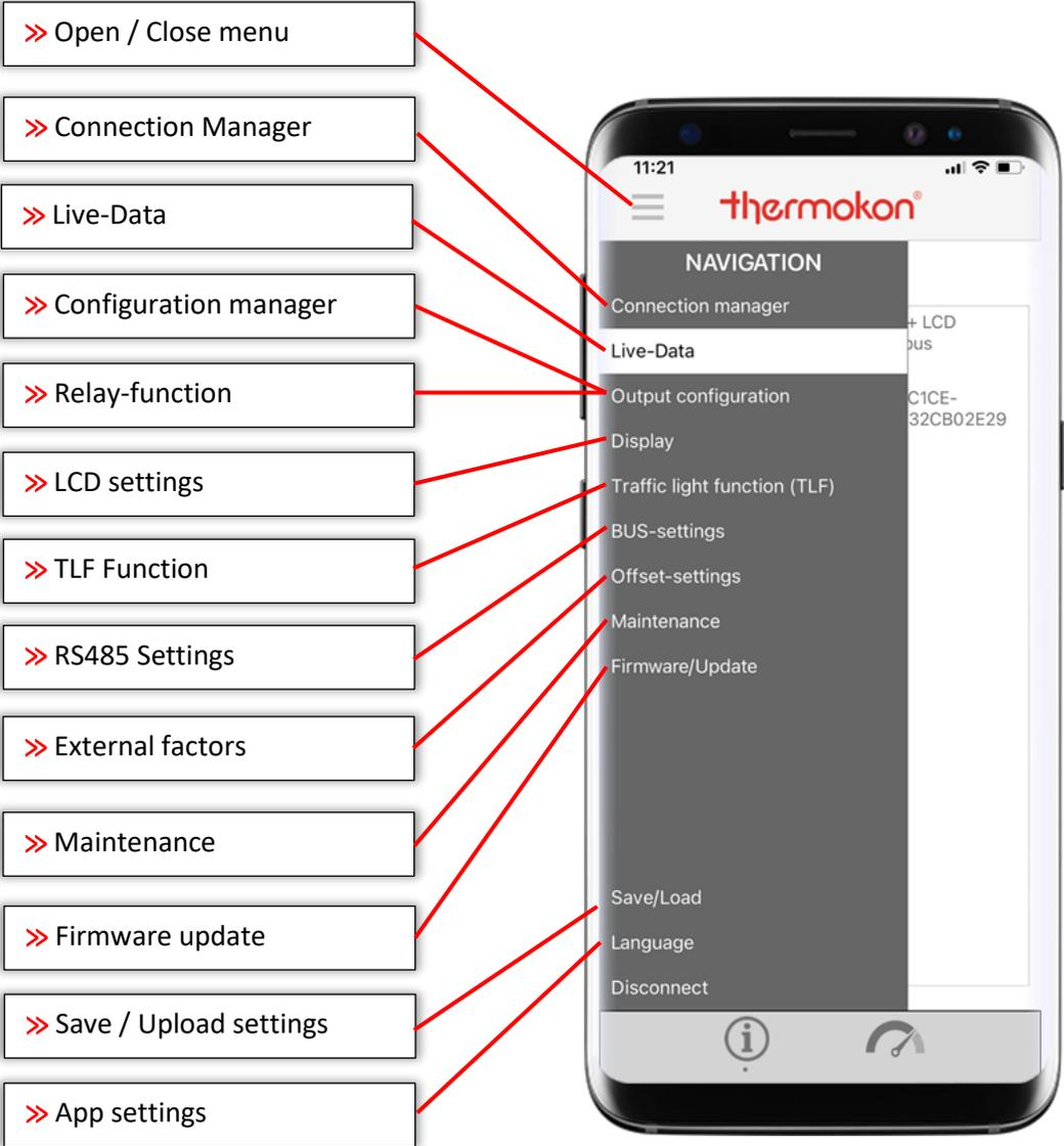
Clicking or tapping on the tiles opens the corresponding submenus. On the following pages, the individual menus and functions are described in detail.
