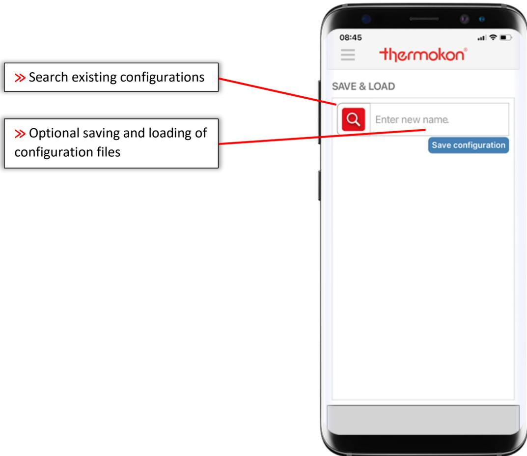
USEapp allows the user to save configurations and re-upload them later. When clicking on **Save configuration**, a new window opens to assign a name to the current configuration and to save it. If USEapp is allowed to access the geo-services of the mobile device, the position can be stored where commissioning has taken place. For the user, for example, an even more precise assignment to the project.
