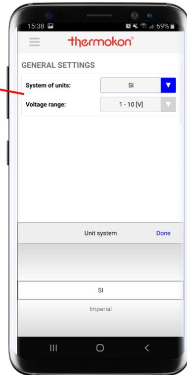
**Measuring system:** Use this drop-down menu to switch between the international (SI) and imperial system of units (Imp). The changeover refers to all measured variables and output signals of a unit. When changing from SI to IMP, for example, the unit of Celsius (°C) in Fahrenheit (°F) for a temperature sensor or the unit of Pascal (Pa) in Inch Water Column (inchWC) for a differential pressure sensor is adjusted and automatically re-scaled.
