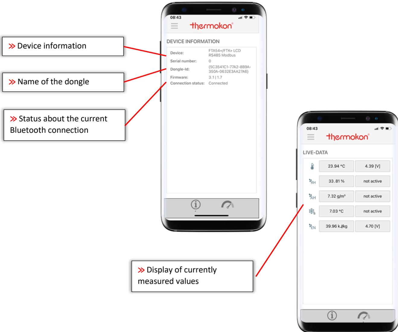
**Device information:** This area appears as a header in all menus and describes device-specific properties. In addition to the name and serial number of the connected device, the Bluetooth dongle ID and firmware version of the base and option PCB are also displayed. The Connection Status field informs the user whether the connection to the sensor is active or disconnected.
