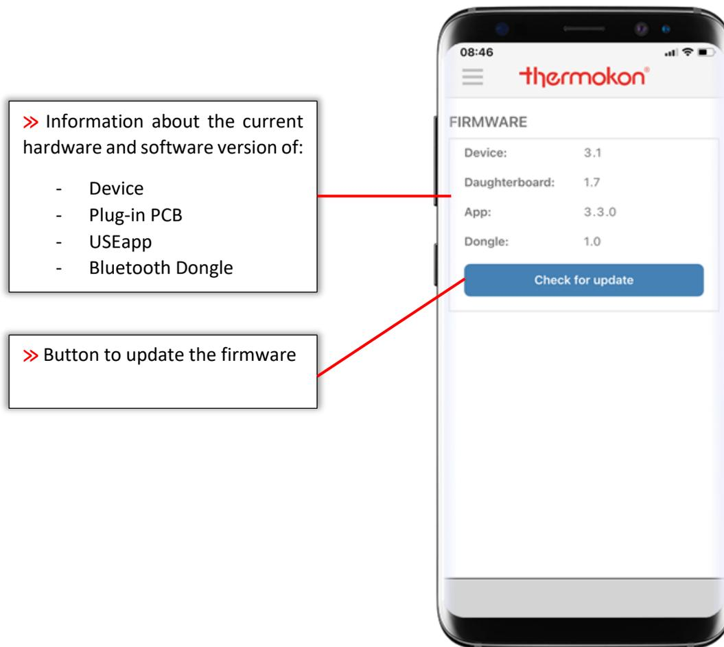
Sensors with USEapp support can be updated in a mounted state. After the connection between the USEapp and the sensor has been established, the app compares the latest software version on the server with that of the sensor. If a new firmware is available for the device, the latest version can be transferred to the device via the **Update button**.
