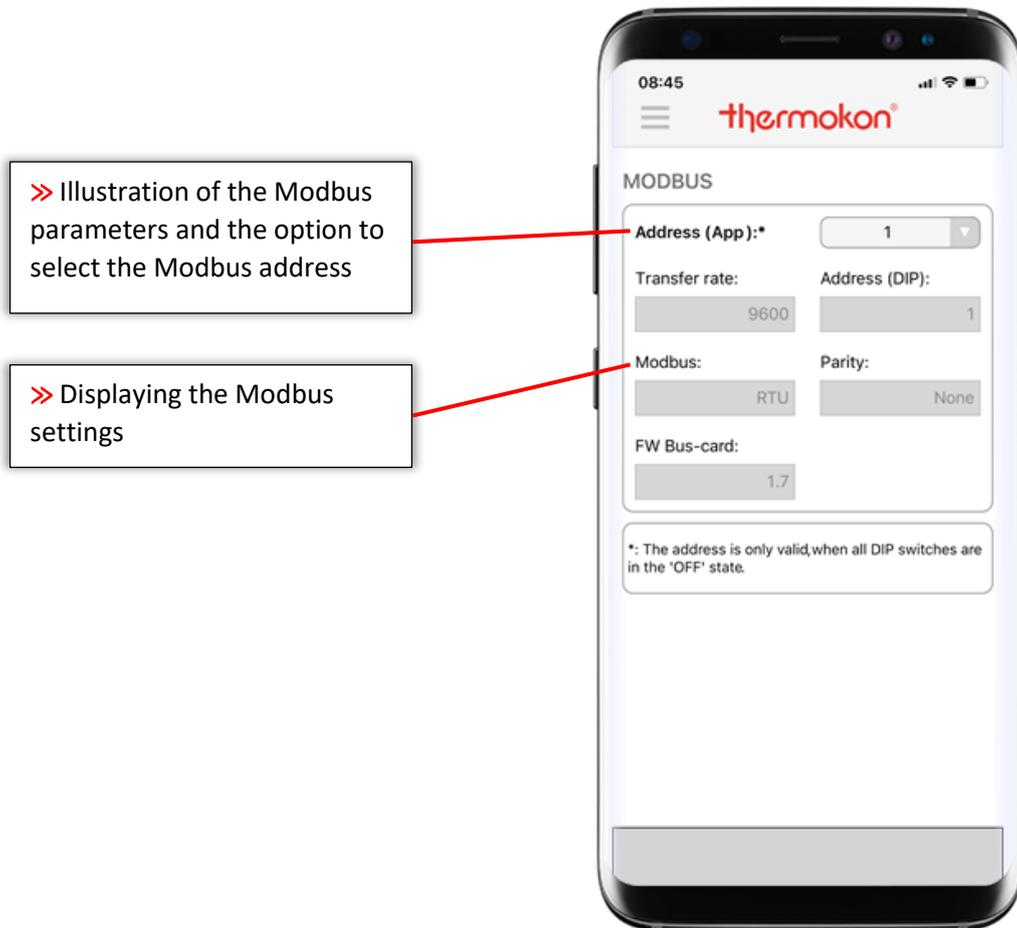
With all Modbus sensors of the USE family, it is possible to assign an address range from 1 to 247. Address assignment from 1 to 31 is possible via the DIP-switches on the circuit board. If this is not sufficient in certain cases, the user can extend the address range up to 247 via USEapp. For this purpose, all DIP-switches for the address range must be set to **OFF**. Using the drop-down menu Address (APP):\* you can now assign an address.
