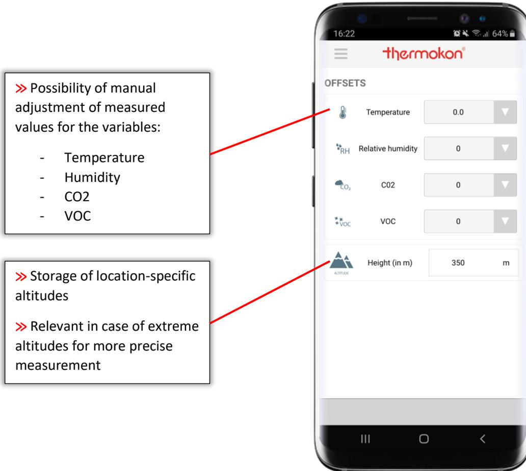
The consideration of external factors that could possibly influence the measurement result is easily done via USEapp. For this purpose, there is the possibility to manually adjust the measured values. In the grey field behind the icon of a measured value, the actual measured value is displayed. An offset can be stored via the corresponding drop-down menu. The possible adjustment ranges are listed in the table on pages 22 and 23.
