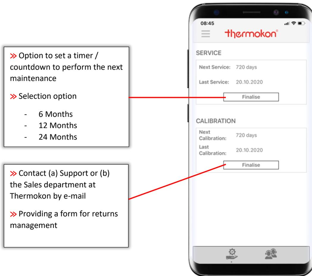
All devices with USEapp support have an integrated operating hours counter. The user can store maintenance and calibration intervals in the sensor via the USEapp in order to be automatically notified by the sensor after a certain period.
