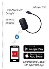
Parameterization with mobile devices via Bluetooth and NOVOSapp. A separately available Bluetooth dongle\* is required (item no. 668262).
