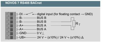
With alternating voltage, the correct polarity must be ensured! Please note the technical data. Don't forget the BUS termination (120 Ω) at the last device of the line! (Not included in delivery)
