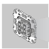
During assembly, ensure the correct orientation (top / bottom) of the key card switch.
