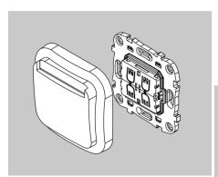
Mount key card switch to the smooth wall surface or flush mounting box using double sided tape or screws. The retaining screws may only be tightened hand tight. The devices are supplied in operational state. Make a flat surface before mounting on rough surfaces. Unevenness can lead to a malfunction of the transmitter. Observe the mounting position of the transmitter during installation. Remove the trim plate from the key card assembly.
