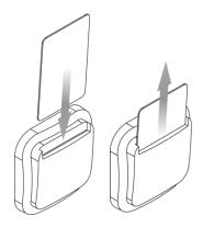
To make sure that the switch information is interpreted correctly at the receiver, it is necessary to learn-in the key card switch into the receiver. This is done automatically by actuation of the key card switch.
