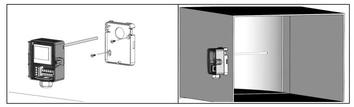
Mounting with immersion pocket or compression fitting for usage in liquid media. Use contact fluid for better heat transfer between sensor and measuring medium.
