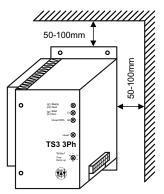
The housing design according to IP 54 (Option) can be mounted in places which are not protected from dust and humidity.
