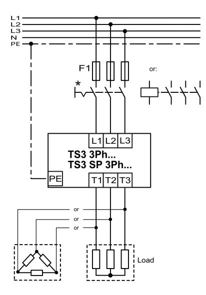
\* For disconnection plug connectiors, fuses, circuit-breakers, load-breakers, residual current devices (RCDs), etc. can be used.
