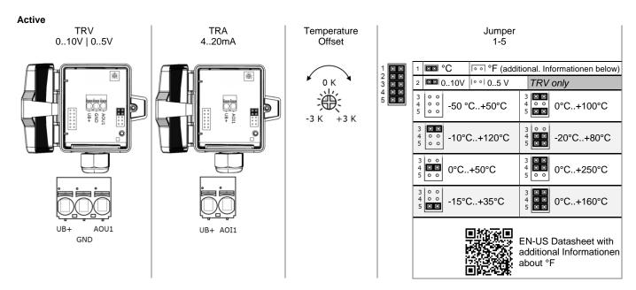
fig. (Measuring range and offset adjustment, default settings: 0 °C..+160 °C | 0 K)
