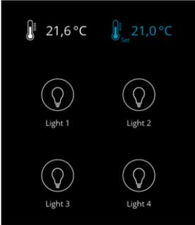
To reduce the risk of burnt-in effects of the screen contents, it is recommended to activate the screen saver. By default, the screen saver switches on 120 seconds after the last interaction.
