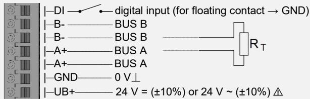
With alternating voltage, the correct polarity must be ensured!
