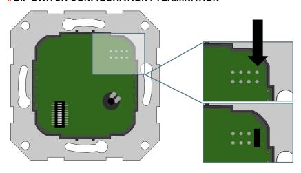
Don't forget the BUS termination (120  $\Omega$ ) at the last device of the line!
