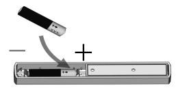
Insert the battery. Pay attention to battery polarity!
