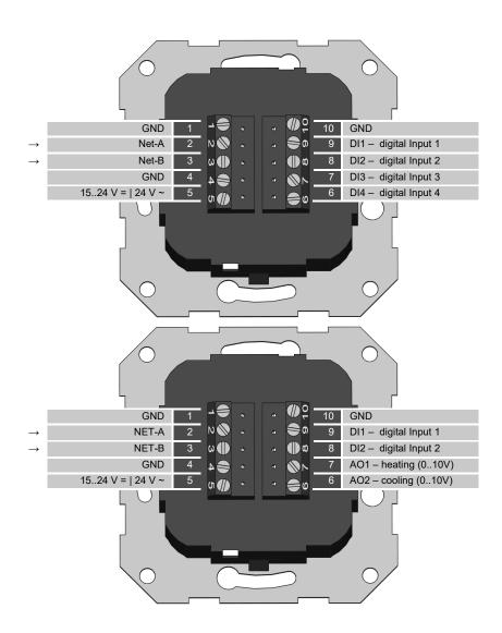
BUS connection type DO2R/DO2T/OVR/OVT  $\rightarrow$  Terminals 2 and 3 on the basic unit.
