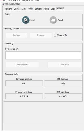
Airconfig can save the configuration of the STC-BACnet IP V4 with a cloud function if required. A subsequent ID change is only possible with a local backup.
