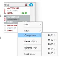
Teached-in sensors can be replaced with identical devices with an identical EEP. (right-click -> replace). This is intended for exchanging / replacing devices without adapting BACnet programming.
