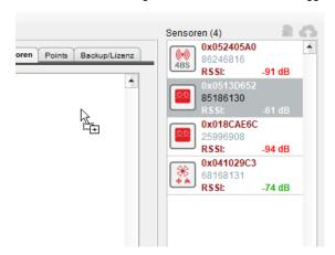
The "Sensors" area shows the EnOcean telegrams that can be converted into BACnet data points. In order to generate data points, the gateway must know the ID and the EEP of the sensor, as this defines how which data point is generated. Therefore, only EnOcean sensors whose EEP has been recognized by the learning telegram or to which an EPP has been manually assigned can be assigned.
