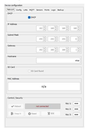
With DHCP, the connection-seeking gateway requests the IP address configuration from a DHCP server.
