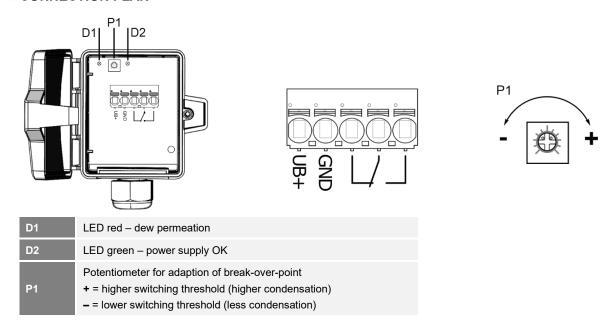
The layout of the relay contacts represents the operation status of "devices connected to power supply, no dew permeation". In this operating state, contacts 3 and 4 are connected to each other. Upon dew permeation or when the operating voltage is switched-off, the relay falls off.
