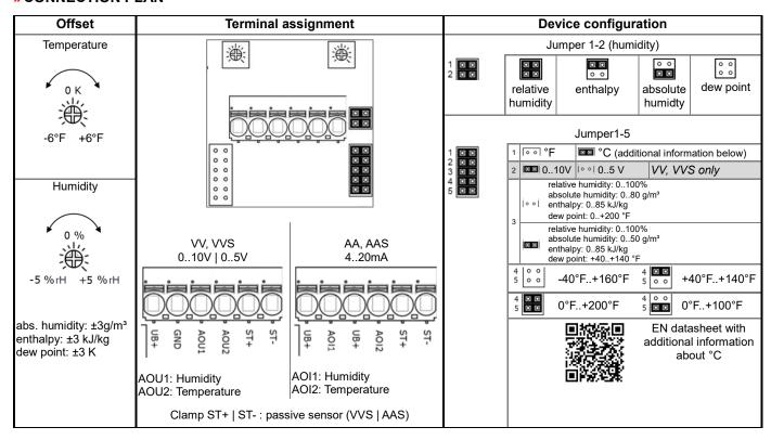
The adjustment of the measuring range is made by changing the jumpers in a de-energized state. The output value of the new measuring range is available after 2 seconds. fig. (Measuring range and offset adjustment, default settings: 0 °F.+200 °F | 0 °F)
