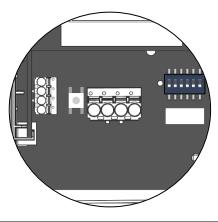
RS485 cable is looped through, connect both cable A+ shields using the enclosed 2-pol. Connect terminal as A+ shown. B-B-B AOU2 GND UB+ volume flow | 0..10 V differential pressure | 0..10 V GND 15..35 V = / 19..29 V ~ IN2 NTC IN2 IN1 NTC
