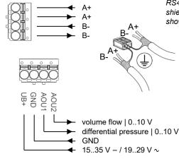
RS485 cable is looped through, connect both cable shields using the enclosed 2-pol. Connect terminal as shown.
