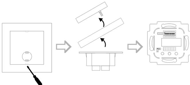
The device is designed for mounting on a flush box. The bus cable is connected to the device by a terminal screw. For pre-wiring, the terminal screw can be drawn from the device.
