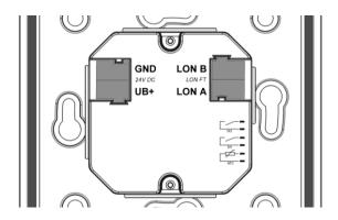
On the side of the lower part of the housing there is a socket connector for connecting up to 2 digital inputs and an NTC10k. The connection is made via a pre-assembled female connector (included in delivery).
