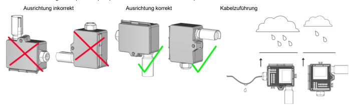
Regardless of the compass direction, the outdoor sensor should not be mounted in the following locations:
