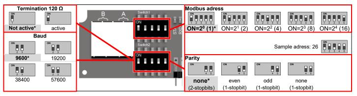
The modbus address of the device is set in the range of 1 ... 31 (binary encoded) using a 5-pole DIP switch. With address 0 via DIP, an extended address range (32...247) is available via USEapp.
