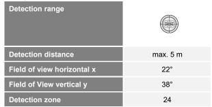
A installation height of 2,5 m results in a detection area of approx. 1x1,7 m, divided into 24 measuring zones.
