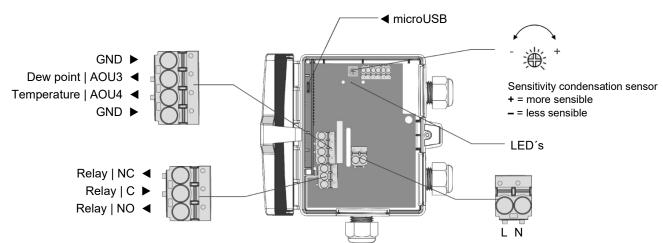
The relay is energized in the operating state (relays NO and C connected). Upon dew permeation or when the operating voltage is switched-off, the relay falls off.
