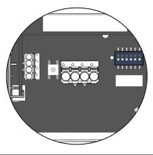
RS485 cable is looped through, connect both cable A+ shields using the enclosed 2-pol. Connect terminal as A+ shown. B-B-B AOU2 GND UB+ volume flow | 0..10 V differential pressure | 0..10 V GND 15..35 V = / 19..29 V  $\sim$ IN2 NTC IN2 IN1 NTC IN1
