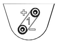
4. Connect pressure tubes to the duct connection pieces
