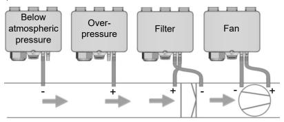
1 Mount the DPA+ mounting base in a suitable location and attach the DPA+. *Note alignment!*
