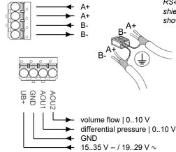
RS485 cable is looped through, connect both cable shields using the enclosed 2-pol. Connect terminal as shown.
