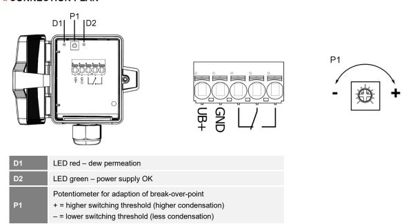
The layout of the relay contacts represents the operation status of "devices connected to power supply, no dew permeation". In this operating state, contacts 3 and 4 are connected to each other. Upon dew permeation or when the operating voltage is switched-off, the relay falls off.
