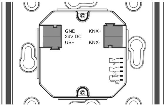
On the side of the lower part of the housing there is a socket connector for connecting up to 3 digital inputs (optional as an NTC10k). The connection is made via a pre-assembled female connector (included in delivery).
