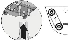
4. Connect pressure tubes to the duct connection pieces
