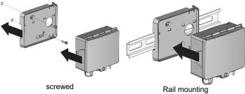
2. Prepare the duct for mounting and mount the duct connection piece.
