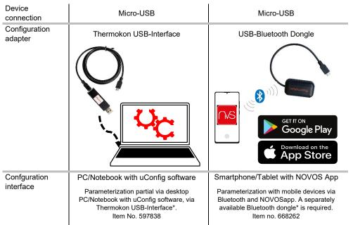
\*Commercially available Bluetooth dongles or USB to Micro-USB adapter cables are not compatible. You need a mobile device that supports at least Bluetooth version 4.1. The configuration app with the corresponding instructions can be downloaded from the Google Play Store or the Apple App Store.
