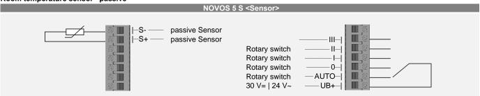
The wiring of the button can be changed via a jumper (see button terminal assignment under configuration). P1 / UB +: Pay attention to the nominal load of the potentiometer of 0.25 W. With 10  $k\Omega$ , for example, 24 V can be regulated.
