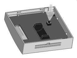
After delivery the room operating unit might be in default shipping mode, in this case press the learn button (<1 second) at the rear of the device [Signal telegramm will be send. SIG -> 0x0F // shipping mode deacticvated].
