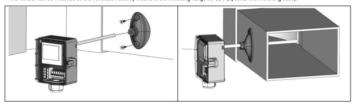
Optional mounting with mounting base (Item No. 631228), please note the installation depth of the sensorpocket. (permissible ambient temperature -35..+70  $^{\circ}$ C)
