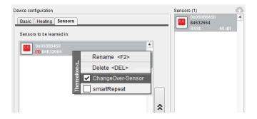
Sensors and devices, within range, are listed on the right side of airConfig. To learn in a specific sensor simply drag and drop the (activated) symbol into the sensors input tab of the STC-DO. The Sensor's (EEP) type must be known to be assigned correctly through activation of the sensor or switch. The sensor type is coded in the EEP, which is included in the sensor's LRN telegram.
