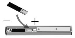
Insert the button cell in the mounting bracket.
