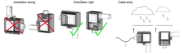
Regardless of the direction of the compass, the outdoor sensor should not be installed in the following locations:
