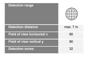
A installation height of 2,5 m results in a detection area of approx. 4,9x4,9 m, divided into 32 measuring zones.
