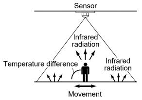
This sensor detects changes in infrared radiation that occur when a person (or object) whose temperature differs from the environment moves.
