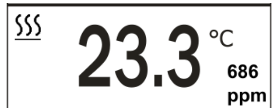
Picture 15 Display of controller mode and humidity or CO2 value
