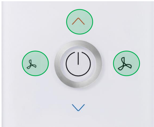
Picture 2 Key combination Fan coil type for invoking parameter menu
