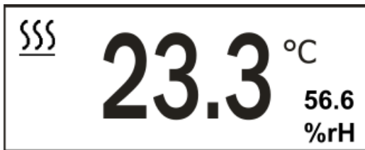
Picture 15 Display of controller mode and humidity or CO2 value
