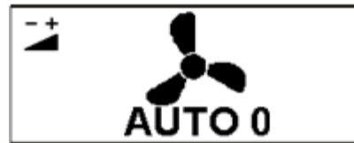
Picture 18 Display of fan coil stage adjustment
