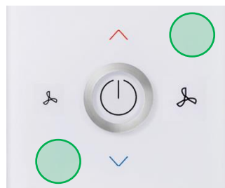
Picture 25 Key combination for resetting to factory settings SCD41
