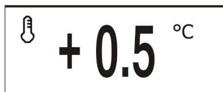
Picture 17 Display of set point adjustment
