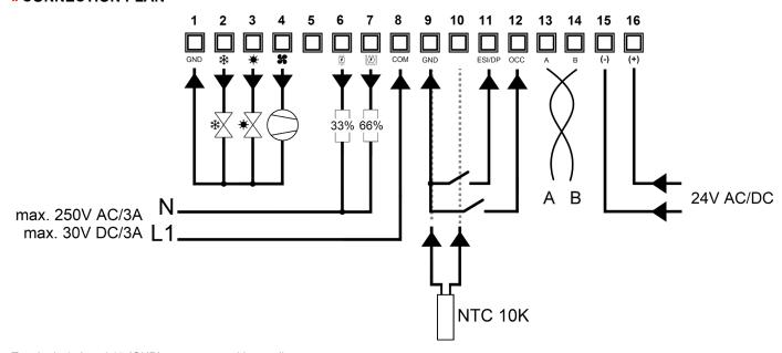
Terminals 1, 9 and 15 (GND) are connected internally.
