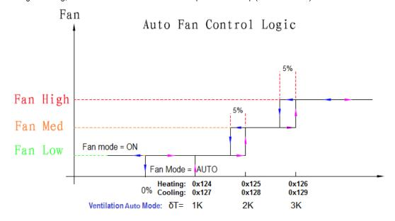
The analog 0..10 V output for the EC fan in automatic mode outputs the voltage value according to the control value of the controller. For manual switching, the following voltage values apply to the EC output:
