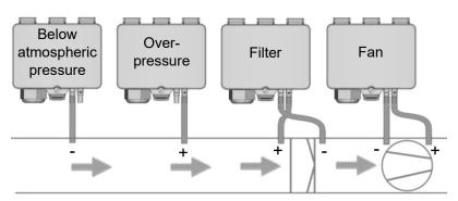
1 Mount the DPA+ mounting base in a suitable location and attach the DPA+. **Note alignment!**
