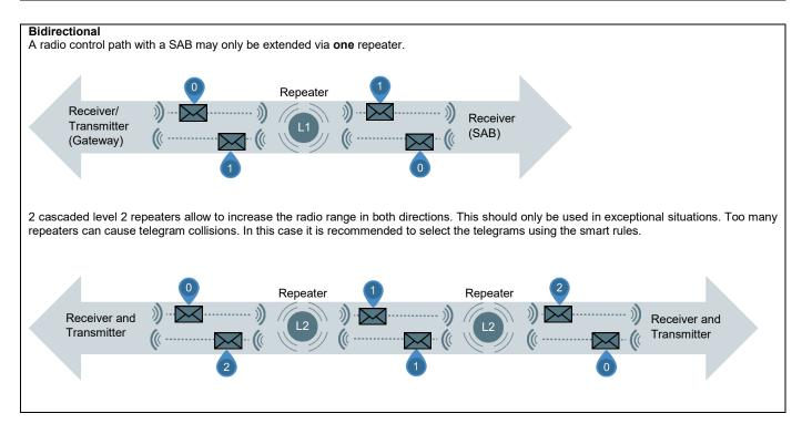
When planning the radio range, it should be ensured that perfect reception is guaranteed at the receiver location. A buffer of the signal attenuation should be considered for a possible later furnishing of the buildings.
