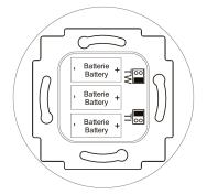
The SR-MDS BAT is battery powered, a wired connection is not necessary. Remove the cover from the backside of the device to insert/exchange the batteries.
