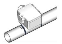
For detection of water condensation, the sensor must be mounted on the coldest point of the medium. Please ensure a good thermal contact to the measuring medium. A thermal connection between sensor und medium with heat conducting paste is necessary. Mounting effects by means of included cable ties (binders). Mounting can be made directly on a pipeline.
