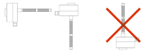
Condensed water must not get into the interior of the enclosure.
