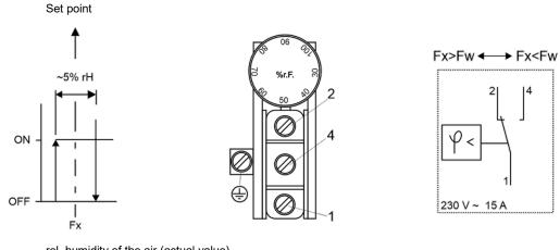
Fx Fw rel. humidity of the air (actual value) humidity adjusted with the wheel (set point)
