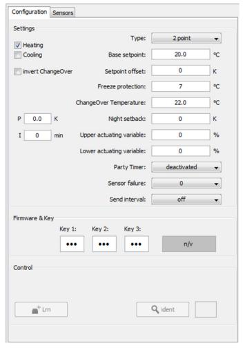
**Controller Type** can be set to 2-point control or proportional control (Plloop) with PWM for thermal actuators.
