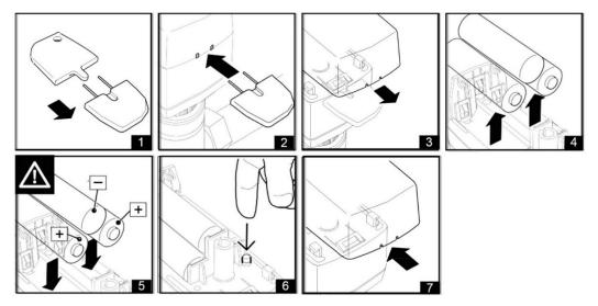
**NOTE** - Insert the batteries with the correct polarity marked in the battery compartment. Only use alkaline batteries (type: AA, LR6 1,5 V). Do not use rechargeable batteries.
