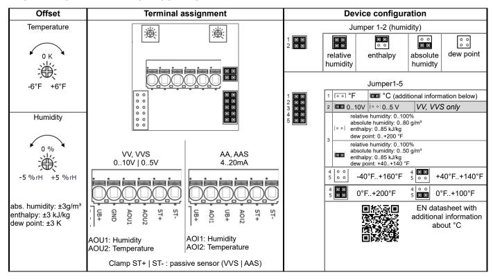
The adjustment of the measuring ranges is made by changing the jumpers in a de-energized state. The output value of the new measuring range is available after 2 seconds. fig. (Measuring range and offset adjustment, default settings: 0 °F.+200 °F | 0 °F)
