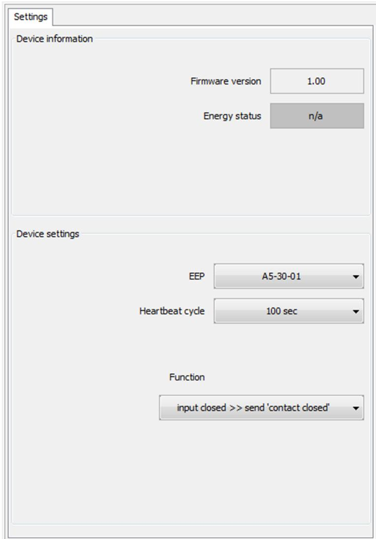
The device information shows the installed **Firmware version** and the current **Energy status** of the device. It is necessary to ensure that the device is full charged or a battery is inserted. The Energy status must be **OK** to configure the device.
