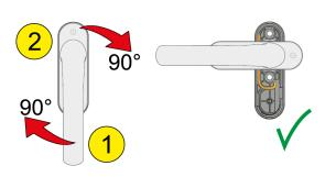
Put the window handle in the  $90^\circ$  position and rotate the cover by  $90^\circ.$
