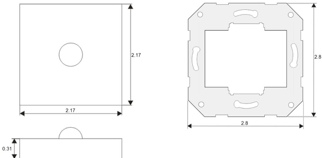
Notice: Outside dimensions are depending on the frame used of the respective switch ranges
