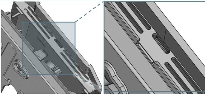
Fix the upper part of the housing on the underside with the screw
