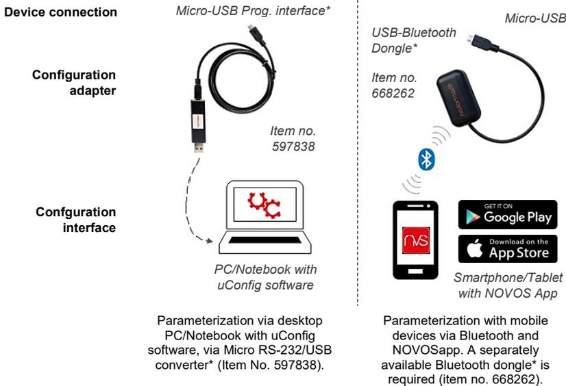
\*Commercially available Bluetooth dongles or USB to Micro-USB adapter cables are not compatible. You need a mobile device that supports at least Bluetooth version 4.1. The configuration app with the corresponding instructions can be downloaded from the Google Play Store or the Apple App Store.
