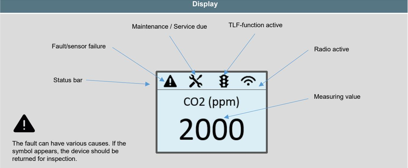
The fault can have various causes. If the symbol appears, the device should be returned for inspection.
