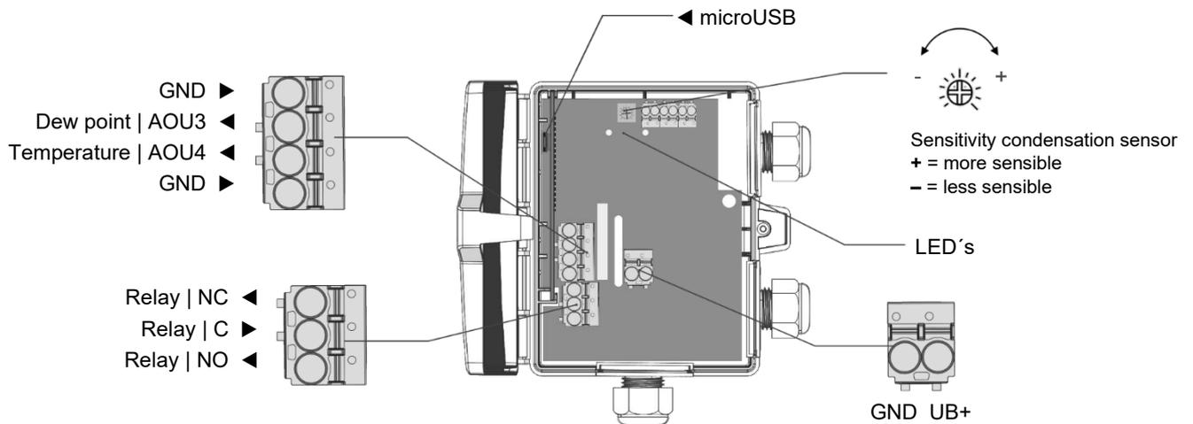
The relay is energized in the operating state (relays NO and C connected). Upon dew permeation or when the operating voltage is switched-off, the relay falls off.
