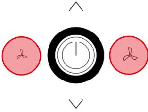
Setpoint change (setpoint range  $\pm 3\text{ }^{\circ}\text{C}$ , default, configurable).
