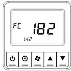
The device information (version and type number) are displayed on the start screen for a short time.
